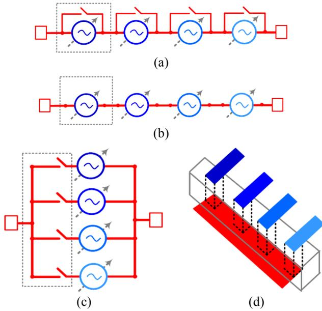
**Fig. 5:** (a) Series switching multi-geometry multi-mode reconfigurable resonator bank using explicit switch for reconfiguration, (b) Series switching multi-geometry multi-mode reconfiguration using short circuit mode of individual resonator, (c) Parallel switching multi-geometry multi-mode reconfigurable resonator, (d) Phase-change via based switching array structure for parallel switching reconfigurable resonator.
