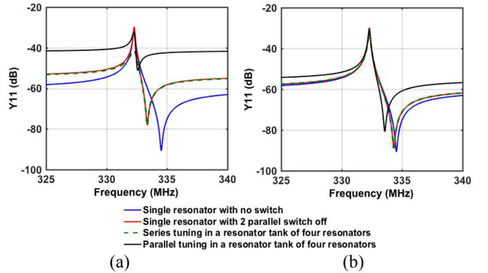
Fig. 8: Admittance plot in Cadence for different switching approaches with PCM via switch (a)  $C_{OFF}=1\text{pF}$ ,  $R_{ON}=15\Omega$  (b)  $C_{OFF}=0.1\text{pF}$ ,  $R_{ON}=2\Omega$ .
