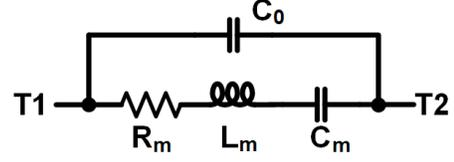
**Fig. 3:** Butterworth Van Dyke Model of AlN resonator.
