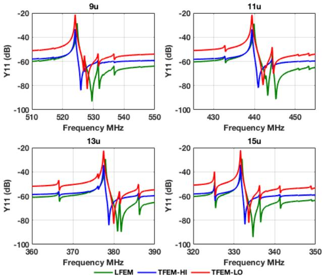
Fig. 7: Simulated (in COMSOL) resonator admittance response for four different geometries ( $W=9,11,13,15 \mu\text{m}$ ) and three different (LFEM, TFEM-HI, TFEM-LO) modes for each geometry showing the ability to multi-frequency multi-mode reconfiguration.
